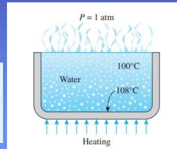
for the boiling of water on a mechanically polished stainless steel surface
