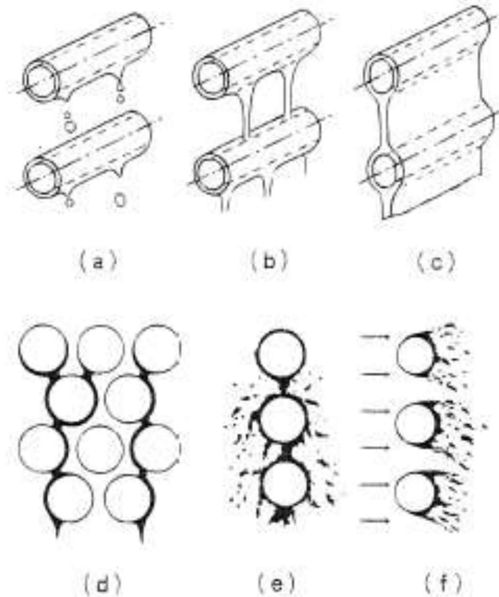
Figure 1. Modes of condensate inundation in horizontal tube banks.
