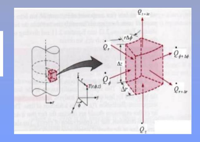
The net rate of heat entering the element in 'r'-direction is:
