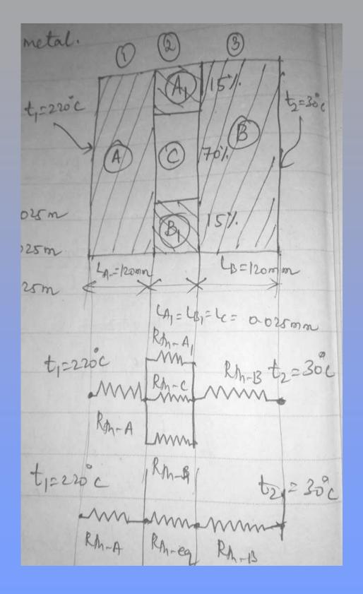
$$\frac{L_{A}}{K_{A}\,A_{A}} + \frac{R_{A1.}\,R_{B1.}\,R_{C1.}}{R_{A1.}\,R_{B1.} + R_{B1.}\,R_{C1+}\,R_{A1.}\,R_{C1.}} + \frac{L_{B}}{K_{B}\,A_{B}}$$
