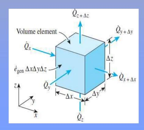
If the directional characteristics of a material are equal / same, it is called as Isotropic material and if kx ‡ ky ‡ kz Anisotropic material
