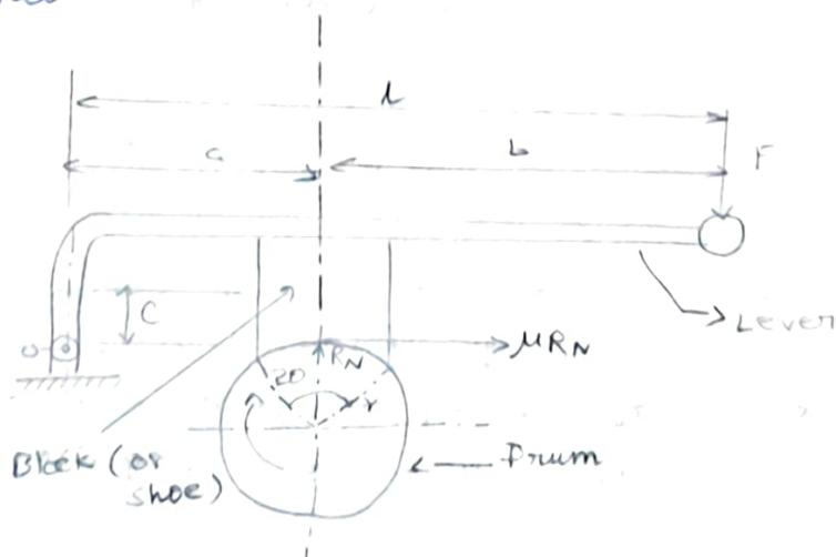
The block is pressed against the drum by a force applied on one end of a lever. The other end of the lever is pivoted on a fixed fulcrum.
