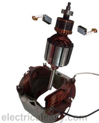
Construction of a universal motor is very similar to the construction of a DC machine. It consists of a stator on which field poles
