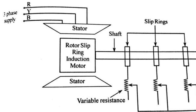
**Figure (4.18) Rotor Resistance Method (or) Additional Resistance Method of speed control**
