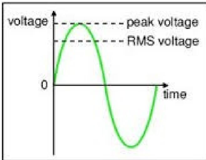
$$rms = \frac{V_{peak}}{\sqrt{2}} \text{ (for an undistorted sine wave)}$$
