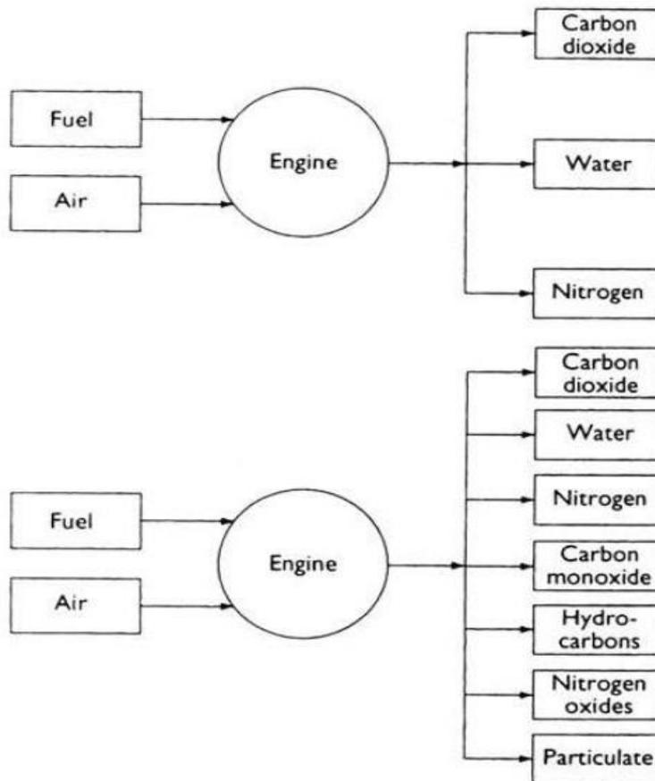
Figure 11. Theoretical results of burning a hydrocarbon fuel and actual combustion results
