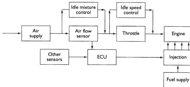
Figure 17. Typical control layout for a fuel injection system
