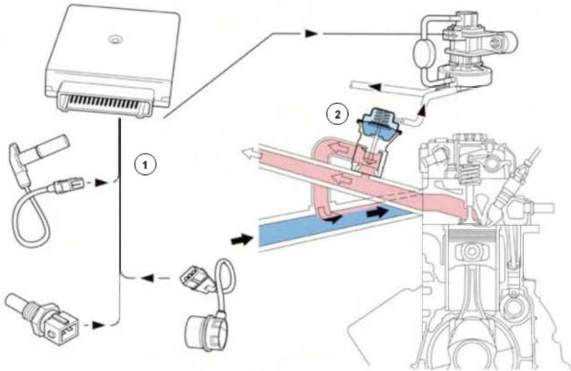
Figure 19. Diesel exhaust gas recirculation (EGR): 1 -ECU and sensors, 2-EGR actuator and control valve
