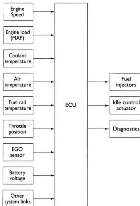
Figure 18. Block diagram of inputs and outputs common to most fuel injection systems
