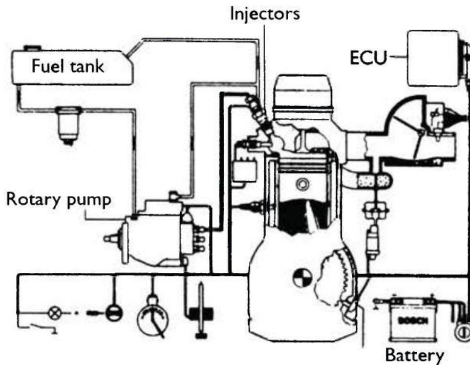
Figure 20. Layout of an electrical diesel control system
