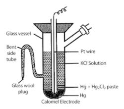
To overcome the limitations of hydrogen electrode, the calomel electrode is developed. This is called the secondary reference electrode. It consists of a glass tube. Pure mercury is placed at the bottom of the tube and is covered with a paste of mercurous chloride. The remaining portion of the tube is filled with a saturated solution of KCl. The bottom of the tube is sealed with a platinum wire.
