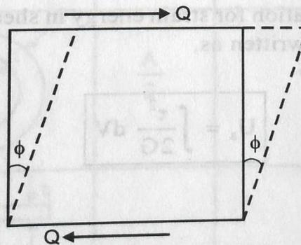
Figure 2.4 Shear loaded structure
