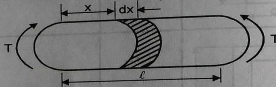
Figure 2.5: Torsional loaded structure
