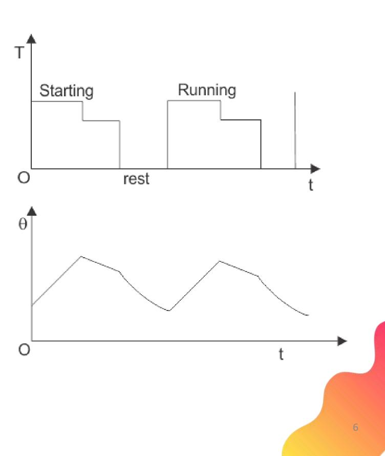
•Continuous Duty with Intermittent Periodic Loading In this type of motor duty, everything is same as the periodic duty but here a no load running period occurs instead of the rest period. Pressing, cutting are the examples of this system.
