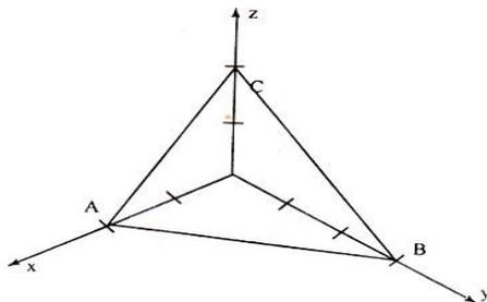
✚ Plane ABC has intercepts of 2 units along X-axis, 3 units along Y-axis and 2 units along Z-axis.
