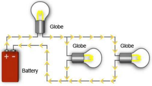
$$\frac{1}{R_{TOT}} = \frac{1}{R_1} + \frac{1}{R_2} + \frac{1}{R_3} \dots \text{etc.}$$
