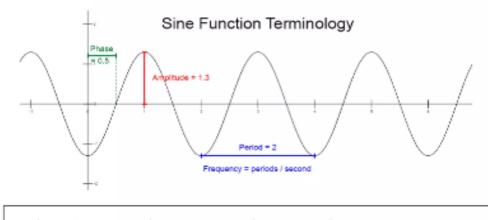
An alternating quantity changes continuously in magnitude and alternates in direction at regular intervals of time. INTRODUCTION TO AC
