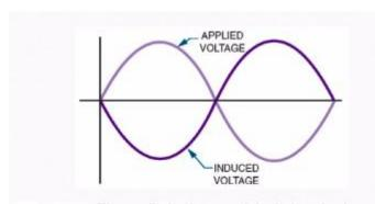
The applied voltage and the induced voltage are 180 degrees out of phase with each other in an inductive circuit.
