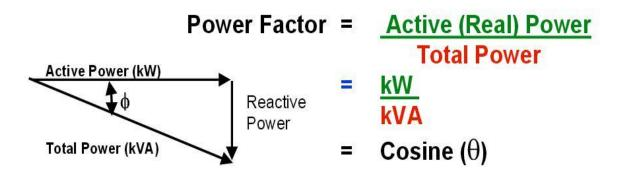
Power Factor is a measure of efficiency (Output/Input)
