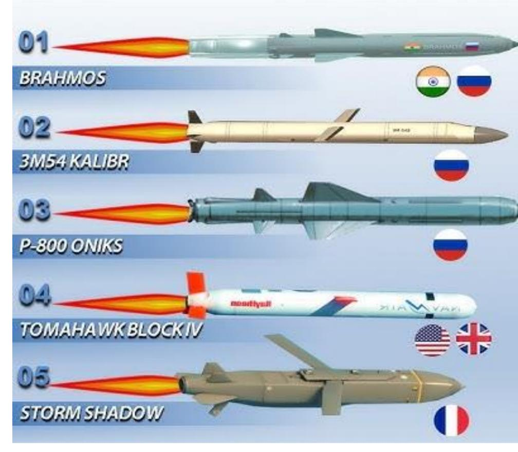
Length: 8.4m/ 28ft Warhead: 200 kg conventional semi-armour piercing nuclear Guidance system: INS, Active radar homing, GPS/ GLONASS/GAGAN Satellite guidance Maximum speed: Mach 3 Operational range: 500 km/ 310 miles
