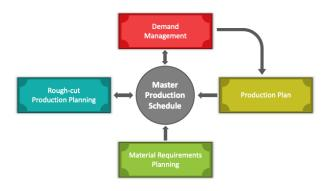
Both APP and MPS are crucial for **effective production planning and control** in manufacturing. APP sets the foundation by aligning capacity with demand, while MPS ensures that the right products are produced at the right time, leading to efficient manufacturing operations.
