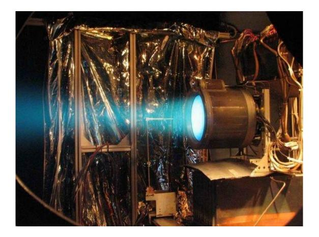
**In electromagnetic thrusters**, a plasma (a special kind of energized gas with ions, electrons, and neutral particles) is accelerated using electric currents and magnetic fields. This plasma is then ejected at really high speeds (from 1000 to 75,000 meters per second!).
