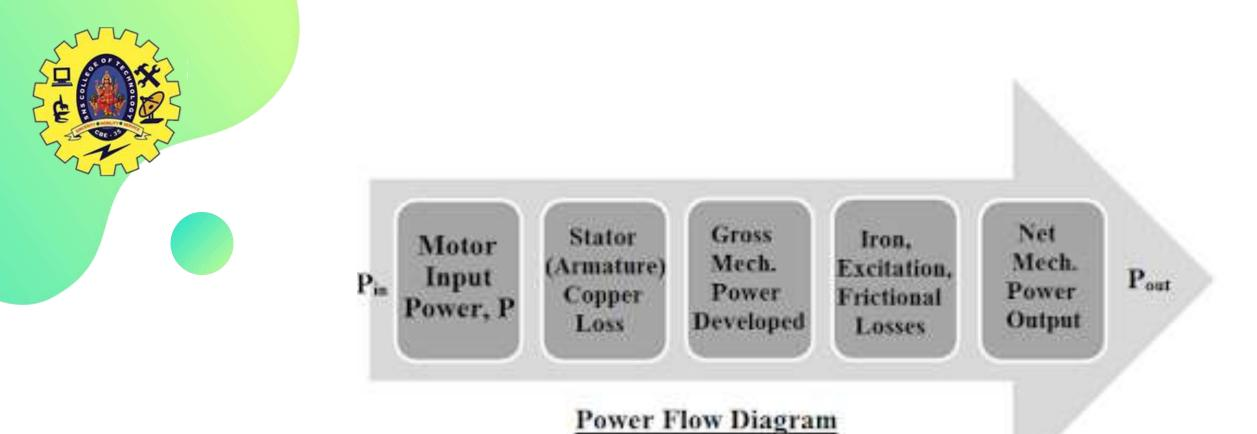
The power developed in a synchronous motor as follows. Motor Input Power, P
