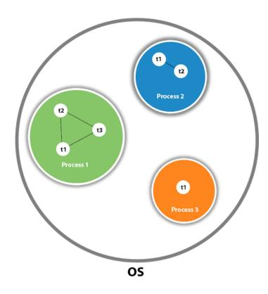
As shown in the above figure, a thread is executed inside the process. There is context-switching between the threads. There can be multiple processes inside the <u>OS</u>, and one process can have multiple threads.
