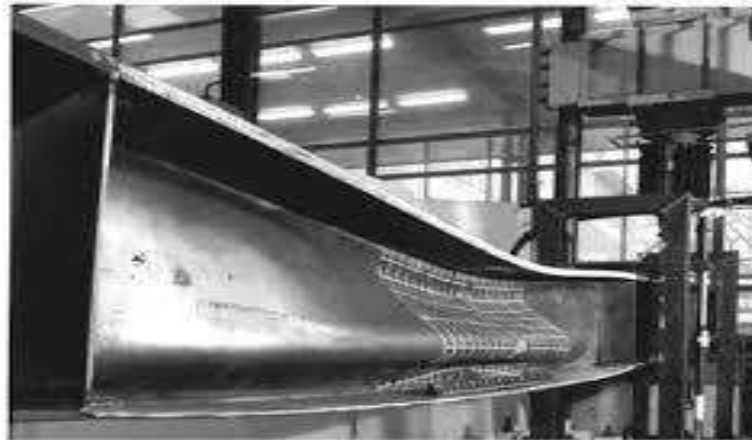
Figure 2. Vertical web buckling.
