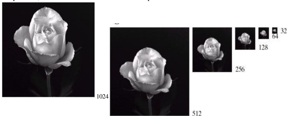
Fig: A 1024 x 1024, 8 bit image subsampled down to size 32 x 32 pixels. The number of allowable kept at 256.
