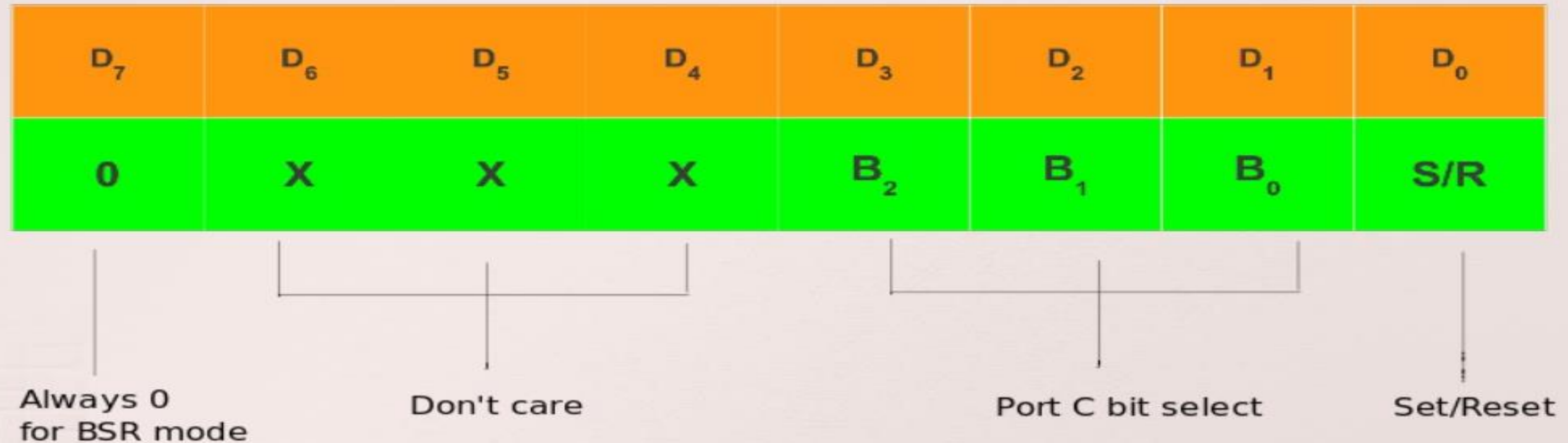
8255 Control Register format for BSR Mode
