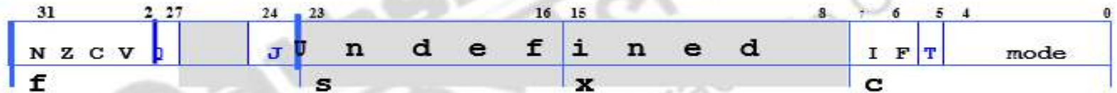
Figure 1.3 Current program status register
