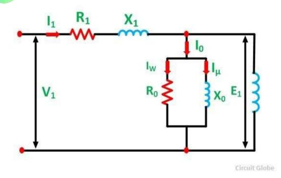
The no-load current I<sub>0</sub> is simulated by a pure inductive reactor X<sub>0</sub> taking the magnetizing component  $I_{\mu}$  and a non-inductive resistor  $R_0$  carrying
