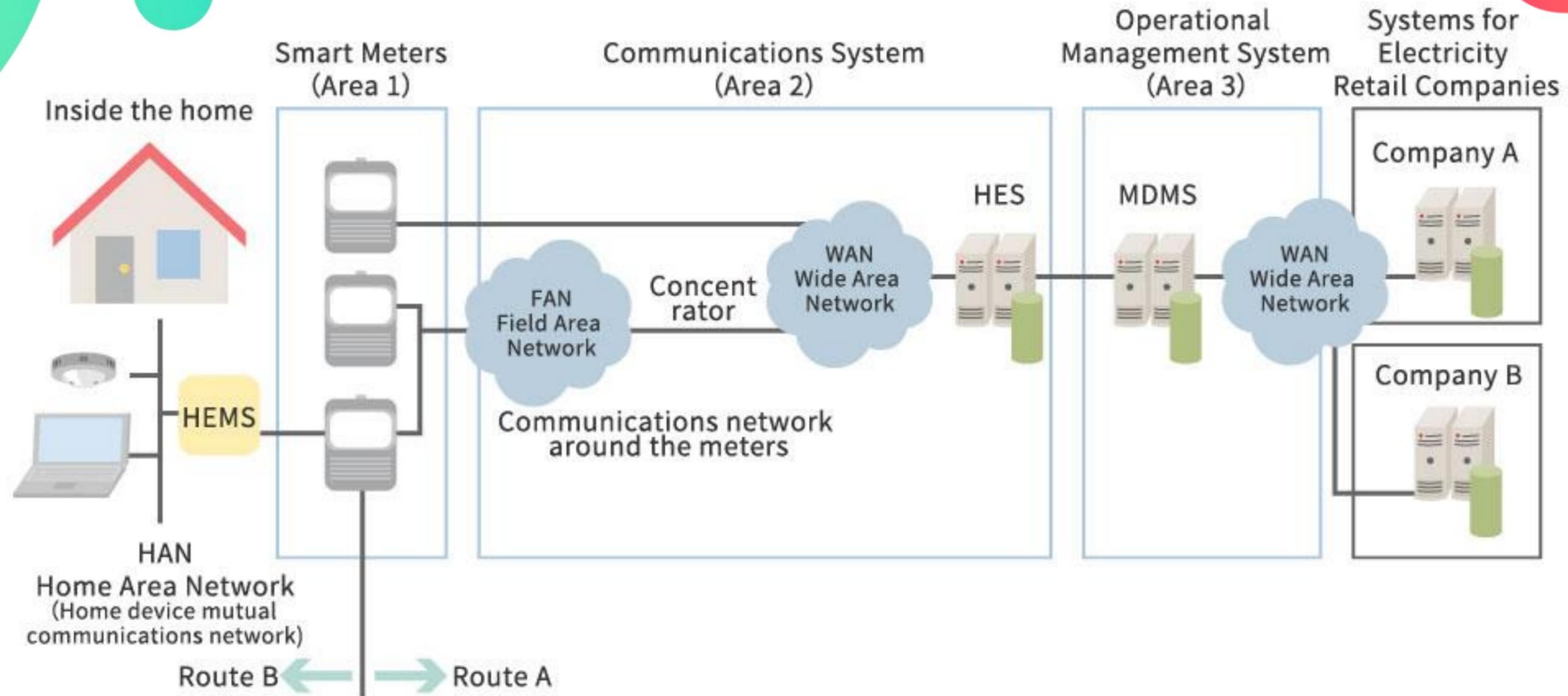
HES: Head-End System (a device that collects data and controls communication)
