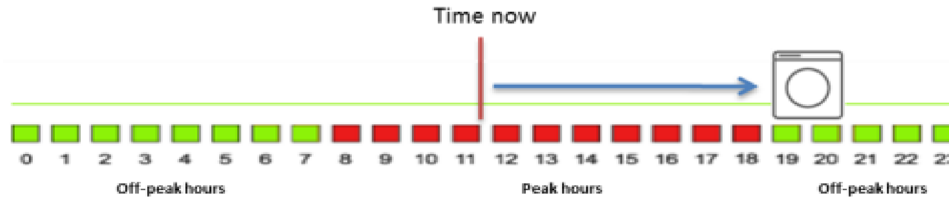
Figure 2: Scheduling of the appliance operation with respect to the price of electricity Source: RSE internal documentation
