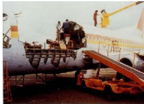
Fig.1.4 Aloha Airlines Flight 243, Boeing 737-200, April 28 1988, Honolulu, Hawaii (undetected cracks in fuselage skin, corrosion in the joint as a result of disbonding)
