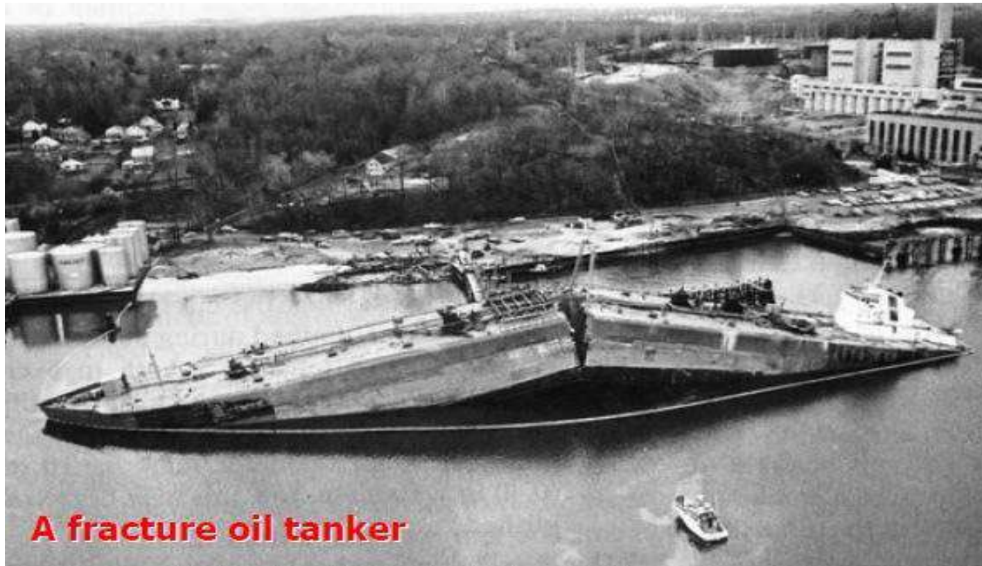
Fig.1.2 An oil tanker that fractured in a brittle manner
