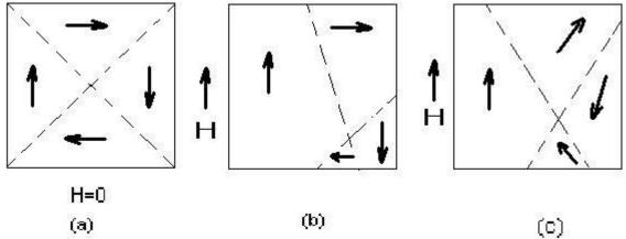
the specimen increases from zero to higher values and attains its maximum value at a point referred to as Saturation Magnetization. When we further increase Magnetic field H there is no further increment in
