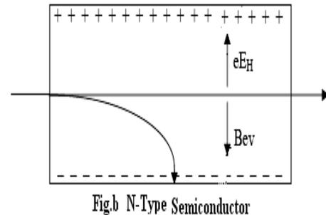
If the sample is an n-type semiconductor majority charge carriers are electrons, these electrons experience a force 'Bev' in downward direction and lower face gets negatively charged and upper face gets positively charged which is shown in fig.b
