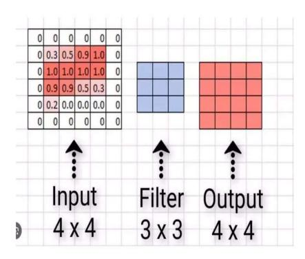
• In the Conv layer, zero-padding is set to 1 to ensure the size of the previous input size.(3x3 kernel)
