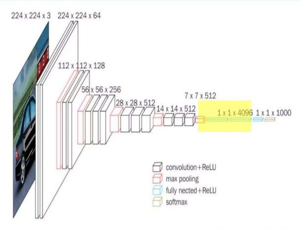
• The training was regularised by weight decay (the L2 penalty multiplier set to 5 X10^-4) and dropout regularisation for the first two fully-connected layers (dropout ratio set to 0.5).
