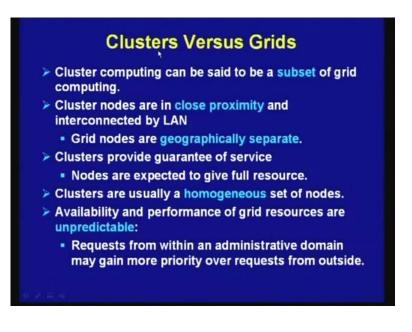
So, here is a comparison between cluster computing versus grid computing, so as I mentioned cluster computing can be said to have a sub set of grid computing. Because, cluster nodes are in close proximity, and interconnected by LAN as I have mentioned, and grid nodes are geographically separate and connected through wide area network or WAN. So, clusters provide guaranty of service, nodes are expected to the full resource on the other hand, clusters are usually heterogeneous site of clusters.
