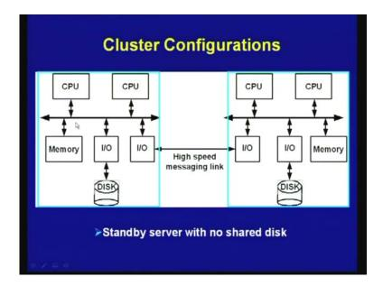
Here you have got two computers shown here, I mean here you have got one you can say, number of processors connected to a shared bus and this is connected to another system, which is also I mean multiple processor and which shared memory. So, these two are shared memory multiprocessors, these two are connected together with a high speed messaging link to work as a cluster.
