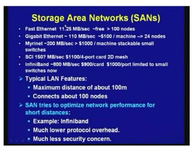
So, these are gives you some components which are use like, the local area network that is been use, you can use high fast Ethernet or Gigabit Ethernet or Myrinet, so these ate type networks that can be used for connecting or InfiniBand, which gives you 100 Megabytes per second. So, you can see these are the rates 11.2 high Megabits per second or 110 Megabits per second or 200 Megabits per second or 800 Megabits per second, so this speed is quite high and distance maximum.
