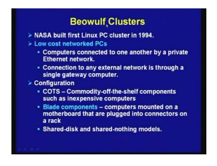
This is an example Beowulf cluster, NASA build first Linux PC cluster in 1994, so it is a low cost network PC's computers connected to one another by a private Ethernet network. So, connection to any external network is through a single gate way computer, and configuration is you are having commodity of self components, such as inexpensive computers. And blade components are use that means, the computers mounted on a mother board that are plugged into connectors on rack.
