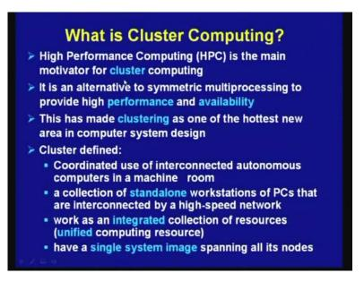
So, as I mentioned high performance computing is the main motivator, and it is an alternative two symmetric multiprocessing to provide high performance and availability. And as a consequence clustering has become a hottest topic in computer system design, you may be asking how do you cluster computing, actually it can defined as coordinated use of interconnected autonomous computers in a machine rooms.
