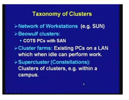
So, let us have a look at the taxonomy of a clusters, one is network of workstations example is Beowulf clusters, where it use COTS PC's that we commonly, I mean commodity of the self PC's with storage network. And you can have cluster forms existing PC's on a LAN, which can hardly can perform work or super cluster or constellation, where you can have cluster of cluster that is within a campus. So, these are possible ways in which you can middle clusters.
