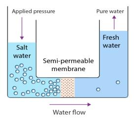
This method is applicable mainly for the desalination of sea water. Sea water and pure water are separated by a semi-permeable membrane made up of cellulose acetate fitted on both sides of a perforated tube. This method is applicable mainly for the desalination of sea water. Sea water and pure water are separated by a semi-permeable membrane made up of cellulose acetate fitted on both sides of a perforated tube.
