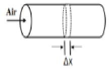
By making material balance on water over a control volume of air of a thickness  $\Delta x$ Water input with air + water transferred to air from the wall by convection = water out with air
