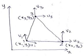
consider a typical est element with nodes 1,2,3, nodal displacements be u, u, u, u, v, v, v, and v.
