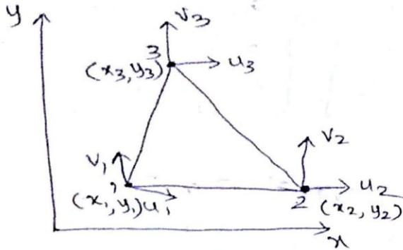
consider a typical CST element with nodes 1, 2, 3, nodal displacements be  $u_1, u_2, u_3, v_1, v_2$  and  $v_3$ .
