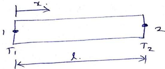
Consider bar element with nodes 1 and 2.  $T_1, T_2$  are the temperature at the respective nodes. So,  $T_1$  and  $T_2$  are considered as DOF of this bar element.
