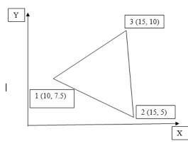
12. For the axisymmetric elements shown in Figure, evaluate the stiffness matrix. The coordinates (in millimetres) are shown in the figures. Let E = 210 GPa and  $\mu$  =0:25 for each element.
