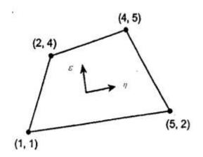
16. Evaluate [J] at  $\xi=\eta=1/2$  for the linear quadrilateral element shown in figure
