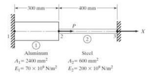
8. The structure shown in figure 1, is subjected to an increase in temperature of  $80^{\circ}C$ . Determine the displacements, stress and support reactions. Assume the following data:
