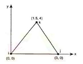
11. Determine the element stresses  $\sigma_x, \sigma_y, \tau_{xy}, \sigma_1$ , and  $\sigma_2$  and the principal angle  $\theta_p$ . The coordinates are given in units of millimetres as shown in figure 4. Assume plane stress conditions. Let E = 210GPa, v = 0.25mm. For the elements given in Figure, the nodal displacements are given as  $u_1 = 2.0mm$ ,  $v_1 = 1.0mm$ ,  $u_2 = 0.5mm$ ,  $v_2 = 0.0mm$ ,  $u_3 = 3.0mm$ ,  $v_3 = 1.0mm$ .
