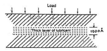
In this case fluid is formed by mixing of hydrocarbon oils and anti-oxidants with long chain polymer so as to maintain viscosity.
