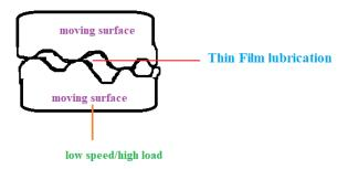
known as boundary film. The co-efficient of friction is around 0.05 to 0.15.
