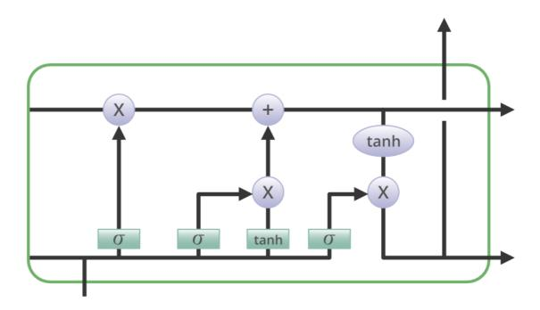
LSTM architecture has a chain structure that contains four neural networks and different memory blocks called **cells**.
