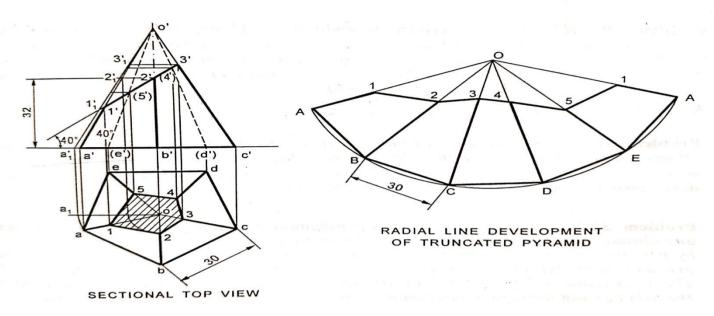
**4**)A Regular Hexagonal Pyramid of side of base 30mm and height 60mm stands with its base on HP such that two of the sides of the base are perpendicular to VP. It is Cut by Plane and Inclined 40° to HP and bisects the axis of the pyramid. Obtain the development of lateral Surfaces of the Truncated Pyramid.
