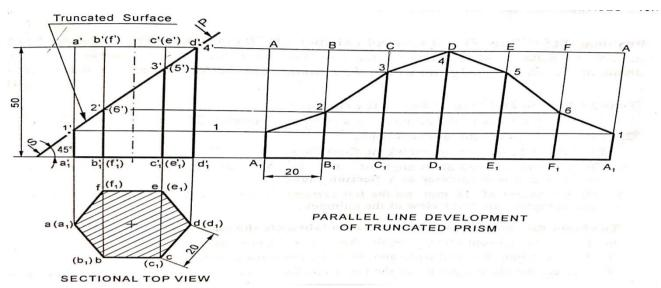
2) A Pentagonal Prism side of base 25mm and Altitude 50mm rest on its base on HP,Such that edge of the base is parallel to VP and Nearer to the Observer. It cut by a Plane Inclined 45° to HP and passing through the Center of the Axis (i)Draw the True Shape of the Section (i)Draw the development of the complete surfaces of the Truncated Prism.
