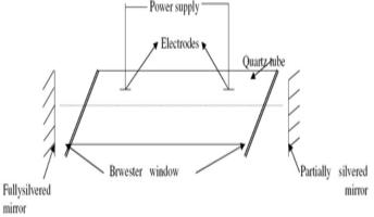
The terminals of the discharge tubes are connected to a D.C power supply. The ends of the discharge tube are fitted with NaCl Brewster windows so that the laser light generated will be polarized. The opticallyplane mirrors fixed oneither side of the normal to its axis as shownin figure. Oneof the mirrors is fully silvered and can reflect all the incident light whereas the other one is partially silvered to get polarized laser beam output.
