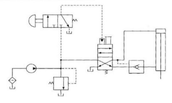
A fail-safe circuit that prevents the cylinder from accidentally falling in the event a hydraulic line ruptures or a person inadvertently operates the manual override on the pilot actuated directional control valve when the pump is not operating.
