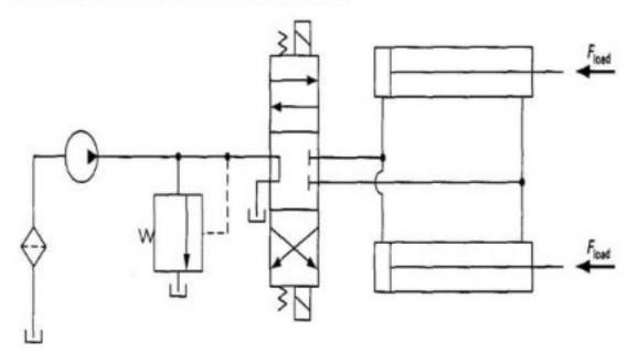
Cylinders hooked in parallel will not operate in synchronization.
