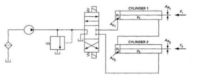
Cylinders hooked in series will operate in synchronization.
