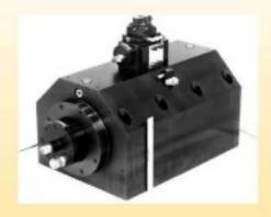
the 3-stage directional servo valves basically consist of the 1st stage control and the 2nd stage in the form of a flow amplifier stage in the 3rd stage for open loop flow control of the main oil flow and an inductive positional transducer whose core is secured to the control spool of the 3rd stage as illustrated in Figure
