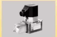
One of the most common types of servo valve is the two stages one. Either a flapper nozzle pilot stage or a jet pipe stage can be used in conjunction with an electric torque motor to control the main spool in the valve as illustrated in Figure.
