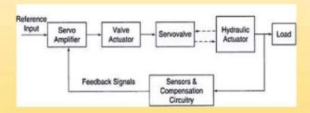
In order to represent the actuator dynamics from the previous equation through a wider frequency range, a second order transfer function is obtained. The transfer function of actuator is the relation between the piston position and the input force can be written as
