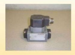
The valve illustrated in the figure is a valve, which employs just one linear force motor (Proportional magnet) to move the spool either side of the central position. The electrical signal from a position transducer is then used for closed loop control of the spool position
