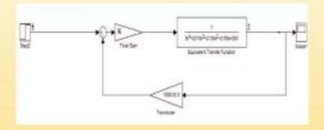
The transfer function of the feedback transducer signal is the relation between the piston displacement and the input voltage v that was found as a constant gain by comparison the ratio between the two parameters.
