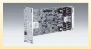
The circuit for the servo amplifier is shown in Figure (4.3), where a smoothed DC voltage between ±22 V and ±28 V is necessary as the supply, and a stabilized voltage of±15 V is then produced from the supply voltage for the amplifier card, this voltage is used for the supply of external actuators such as potentiometers (tapping point at 12c (±15 V) and at 22c (±15 V) and the supply of internal operational amplifiers. Furthermore, two basic function groups should be considered:
