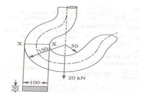
2)A link of S Shape made of diameter 30mm bar shown in figure determine the maximum tensile stress in the link
