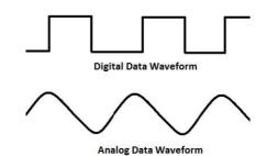
The main function of the modem is to convert digital signal into analog and vice versa. Modem is a combination of two devices – **modulator** and **demodulator**. The **modulator** converts digital data into analog data when the data is being sent by the computer. The **demodulator** converts analog data signals into digital data when it is being received by the computer.
