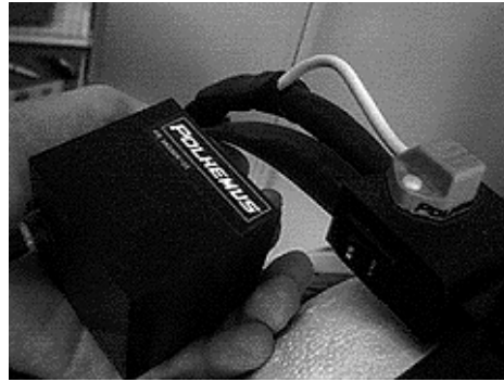
Figure 2.3.1.1. Emitter and receiver units of Polhemus Fastrak.
