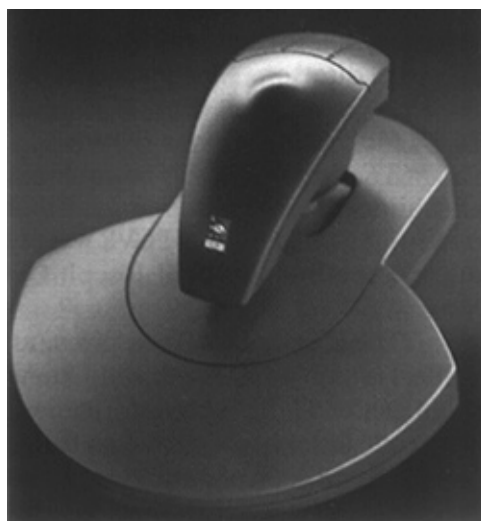
Figure 2.3.4.2. CyberMan from Logitech – desktop 6DOF input device.
