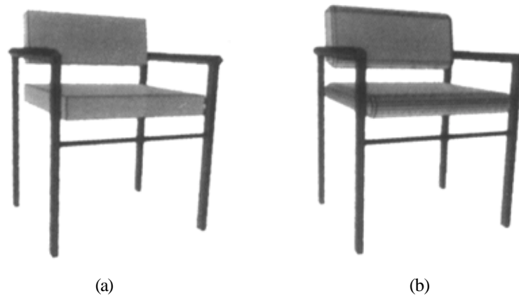
Figure 2.4.1.1. Multiple levels-of-detail of the same object: (a) low LOD, (b) high LOD (from [Funk93]).
