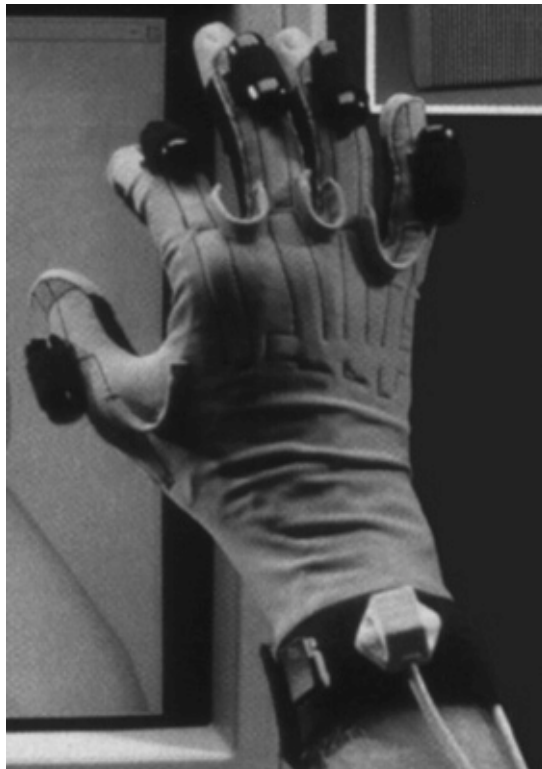
Figure 2.5.2.3. CyberGlove equipped with tactile feedback units.
