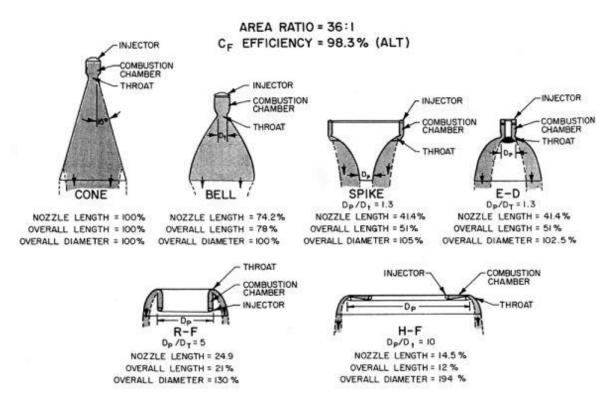
Size comparison of optimal cone, bell, and radial nozzles for a given set of conditions [from Huzel and Huang, 1967]
