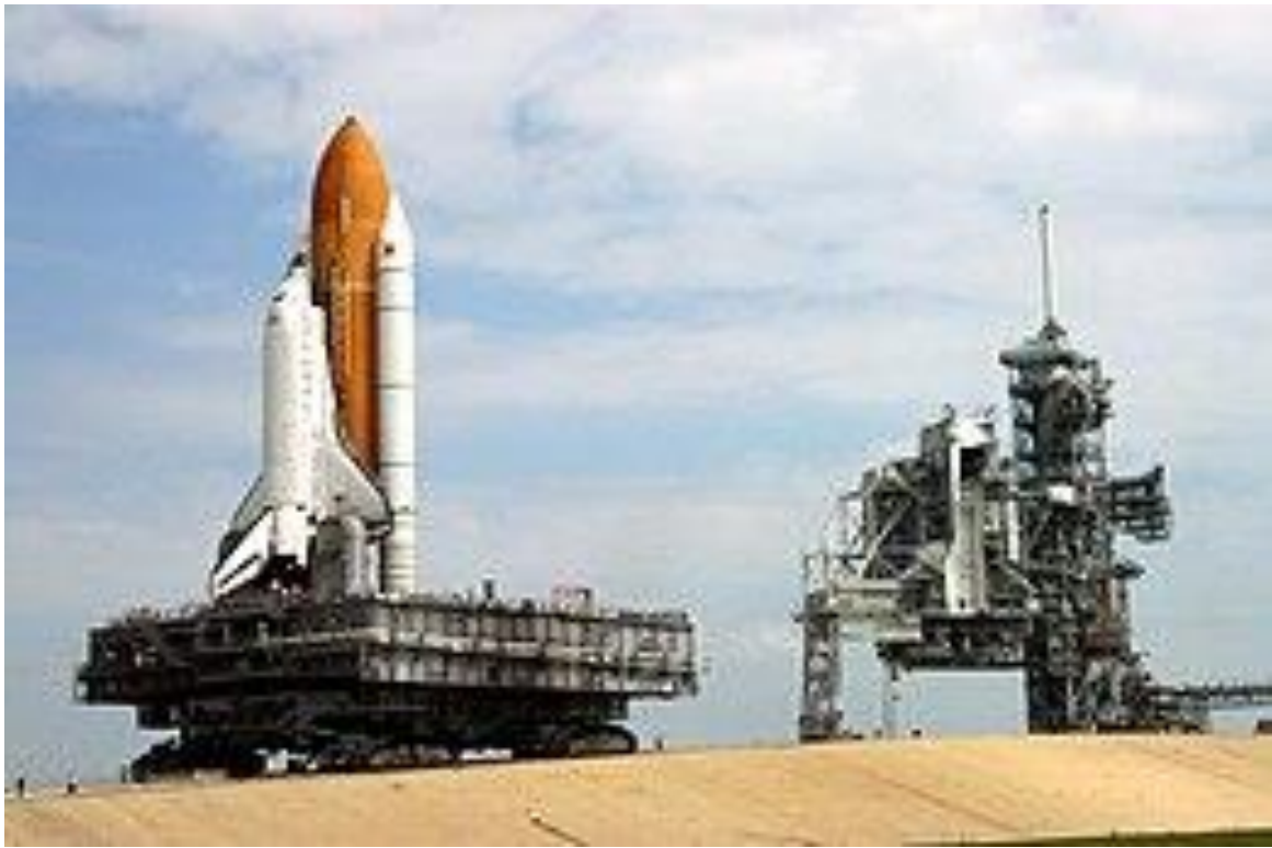
Transport of Space Shuttle and MLP to pad on Crawler-transporter
